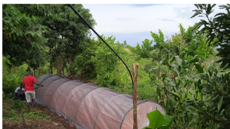
Biodigester covered with greenhouse
